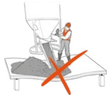
19 ■ Avoid any concrete accumulation while concreting
