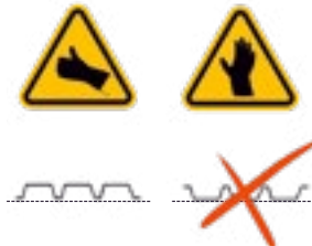
12 ■ Comply with correct orientation of the profile sheet
