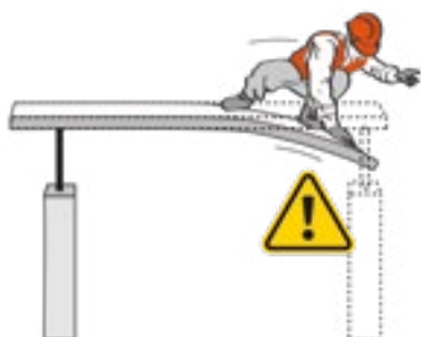
6 ■ Prop where cantilevers are larger than 200mm
