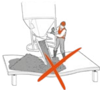
19 ■ Avoid any concrete accumulation while concreting
